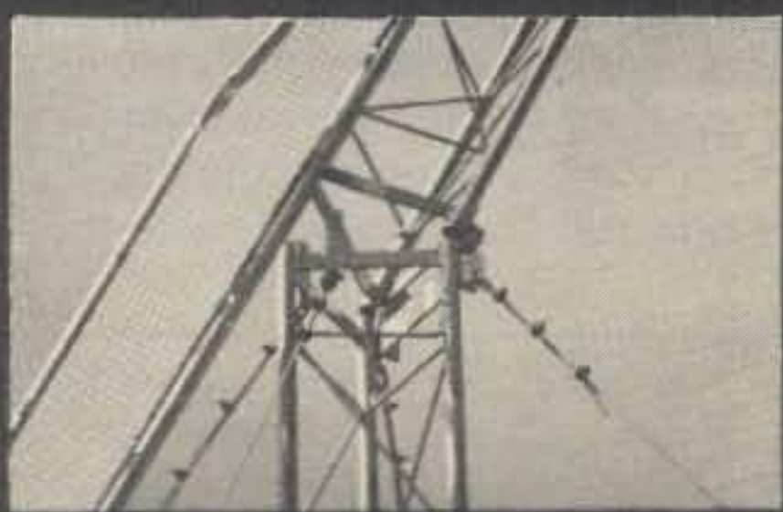
The bottom of the helix showing the radials, capacitor (upper right center of the disc), and the turns.
